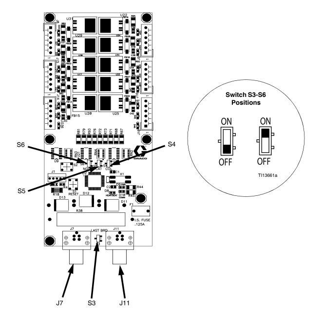
FIG. 16. Color Change Board Switches S3-S6
